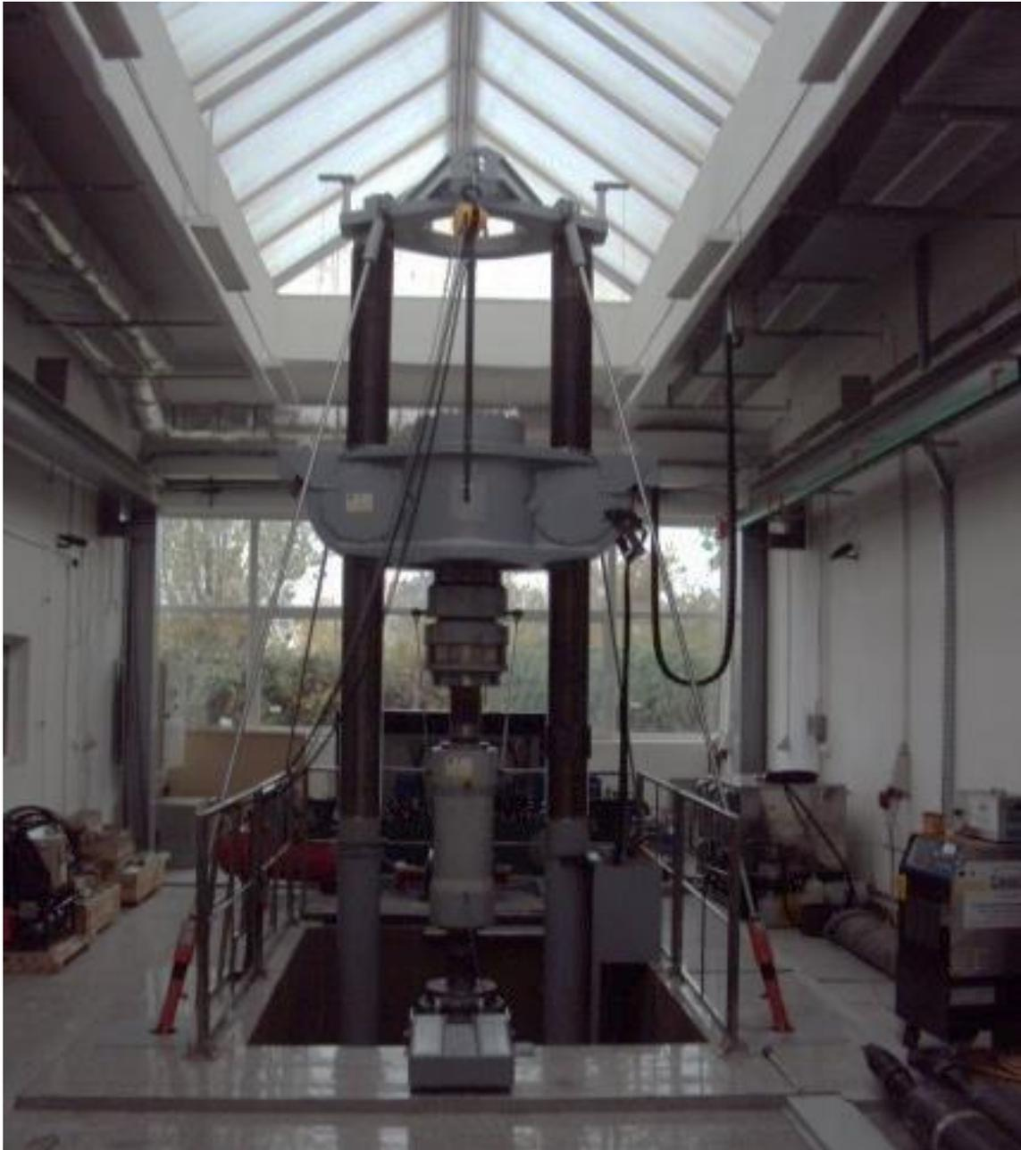
*3. Installation for external pressure (collapse) testing*
